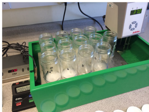
Figure 2022.01C. 2mag Mixdrive 15 submersible magnetic stirrer in custom-built bath with Fisherbrand incubation bottles.
